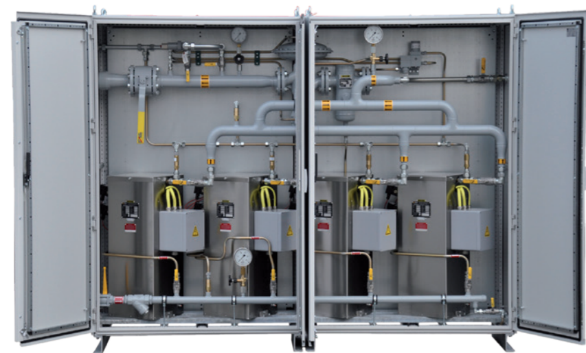
Image left: Version with multiple FAS vaporizers – 2 to 4 pcs. of size 100 kg/hr (26.5 gal/hr) or 170 kg/hr (45 gal/hr). Max. total capacity 620 kg/hr (164 gal/hr) (4 pcs. of size 170 kg/hr (45 gal/hr)).*
