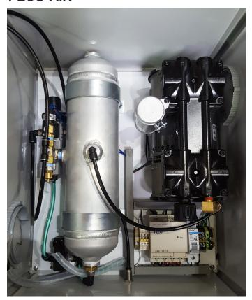
Includes a 1 gallon reservoir to maintain sufficient stored volume of compressed air, to operate multiple pneumatic controls and actuators; up to 21 devices for the ECO-Air, with a 1.5 to 3 second opening time, depending on supply tubing length to control solenoid or actuators. Gauges showing the adjustable regulated output pressure, and operating status give a clear a quick confirmation of the unit status.
