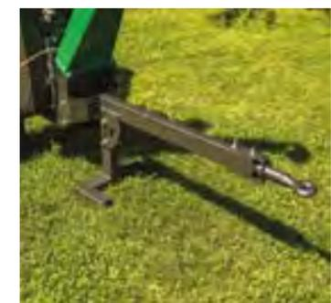
**Supporting Feet with Pivoting Drawbar and Towing Eye**
